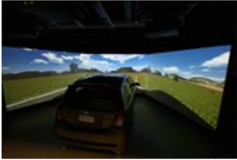
Figure 5. IAD driving simulator
